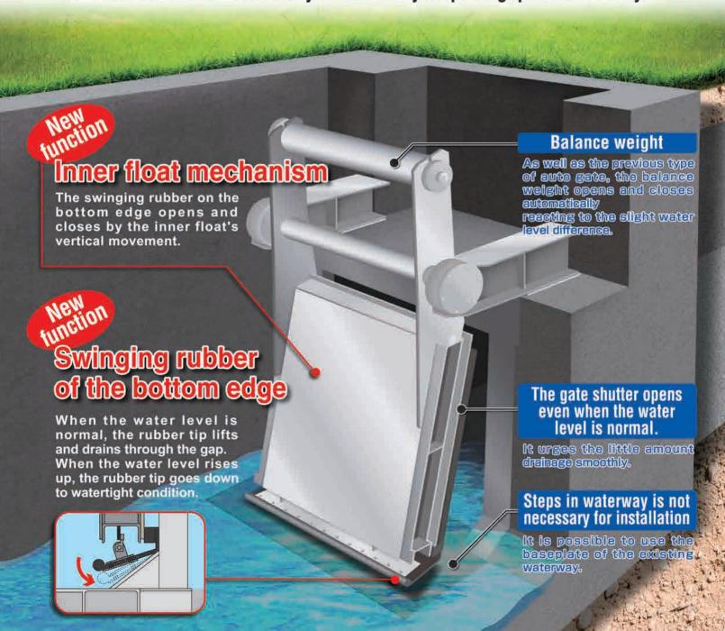
We offer the constructions which utilizes the existing waterway. It realizes the reduction of renovation cost and construction period. Even if the waterway doesn't have any steps, the non-electric auto gate moves rapidly and gives tight waterproof. Adding this auto gate to the existing one is efficient as a belt-and-braces approach.
